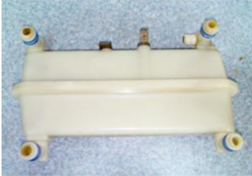
Sealed non serviceable chamber
