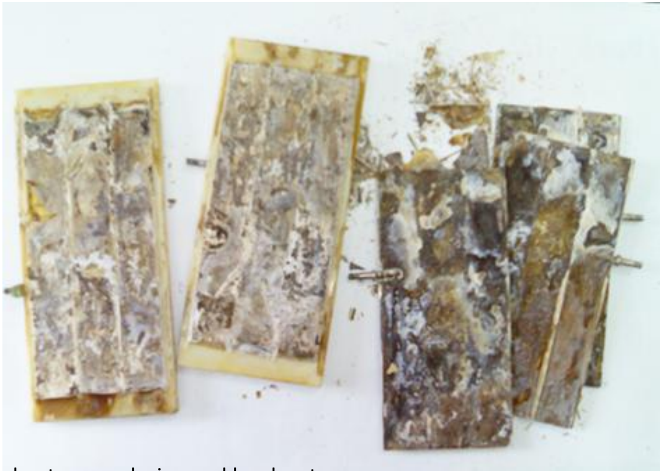
Ruined plates due to poor design and hard water. Not covered under warranty!
